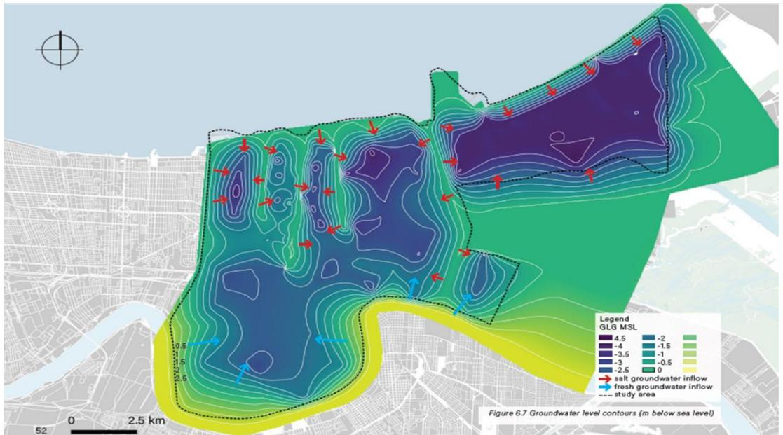
Figure 5-2 Shallow groundwater model generated for New Orleans showing the groundwater flow directions (from areas of light to dark), areas of potential salinization due to saltwater inflow, and areas of freshwater inflow from the Mississippi.
