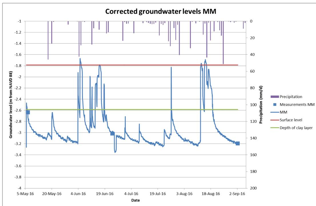
Figure 6-1 Groundwater fluctuation in relation to precipitation events in an observation well in the center of Mirabeau. A number of groundwater monitoring wells are already active within the city. The time series indicates that the groundwater level decreases immediately after a rain event towards the depth of storm drainage pipe and sewer pipe below the streets.
