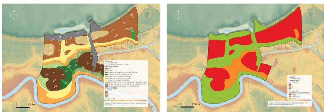
Figure 5-3 (left) shallow soil map displaying types of soil within New Orleans, this information is combined with other to generate the subsidence risk map (right). From the shallow subsidence vulnerability in New Orleans report.
