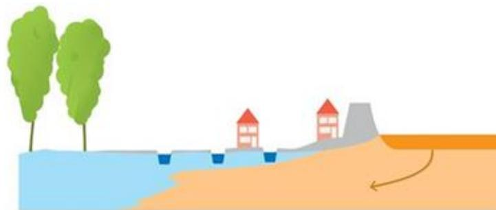
Figure 6-4 (c) Stage 3 – Civil structures and water management practices begin to transform the local ecosystem, reclaiming land by draining a section of the cypress swamp and inducing a flow reversal in the process. Now, the salty groundwater system stemming from Lake Pontchartrain now drains towards the freshwater of the cypress swamp.
