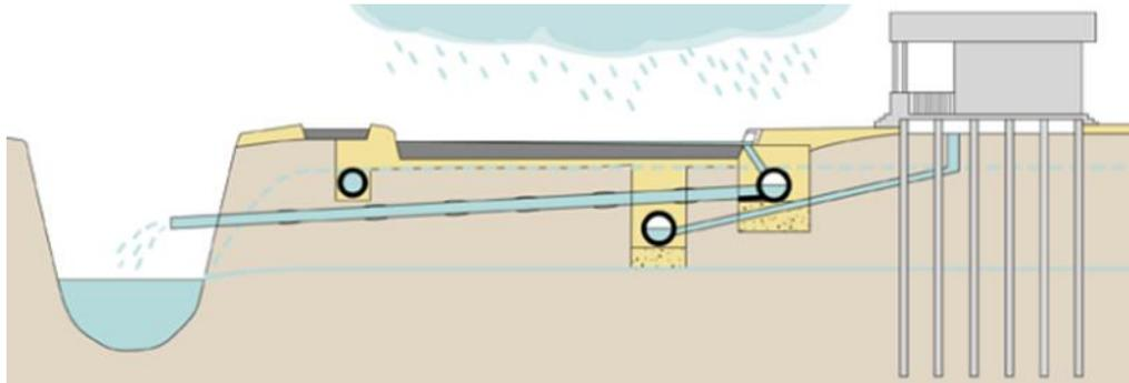
Figure 5-1 Current cross section schematic of the drinking water, sewer and stormwater pipes in New Orleans and associated (low and high) mean groundwater levels.
