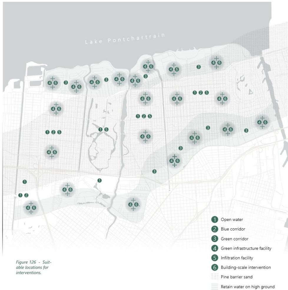
Figure 7-1 Advice for urban water storage based on the geomorphology and drainage networks.
