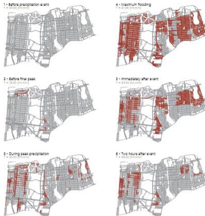
Figure 4-2 The above images were generated with SWMM (Stormwater Management Model) software and shows the effects of a precipitation event on stormwater infrastructure during a given storm (Daan Rooze, 2020).
