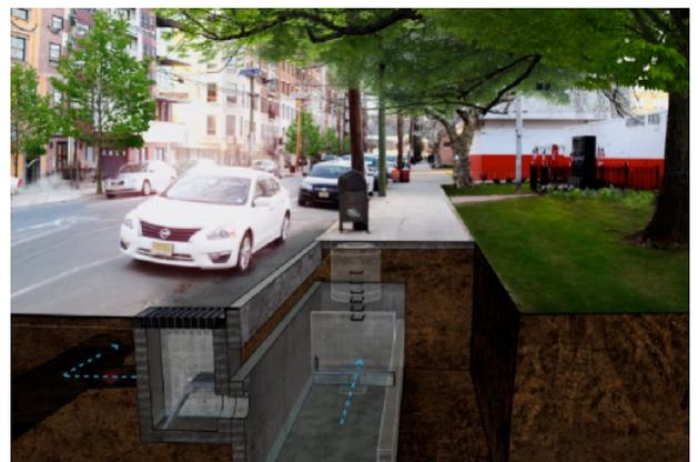
Section view and animation of underground stormwater management systems in Hoboken.
