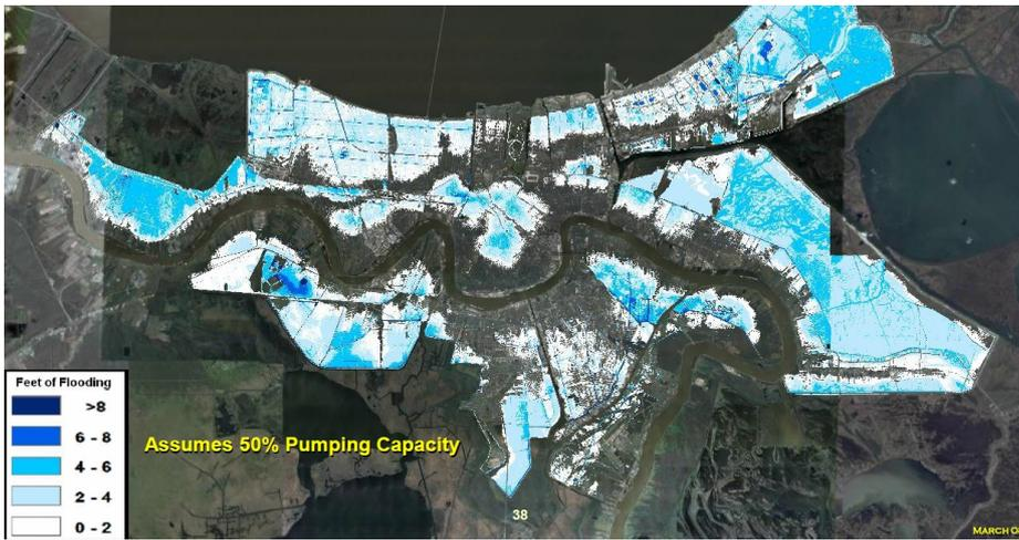
Figure 10: USACE flood scenario for a 500 year surge event showing flood depths in 2 feet steps throughout the greater metropolitan area of New Orleans. In this scenario, the flood infrastructure holds and flooding results from rainfall and overtopping wave action. Pumps are assumed to run at 50% capacity.
