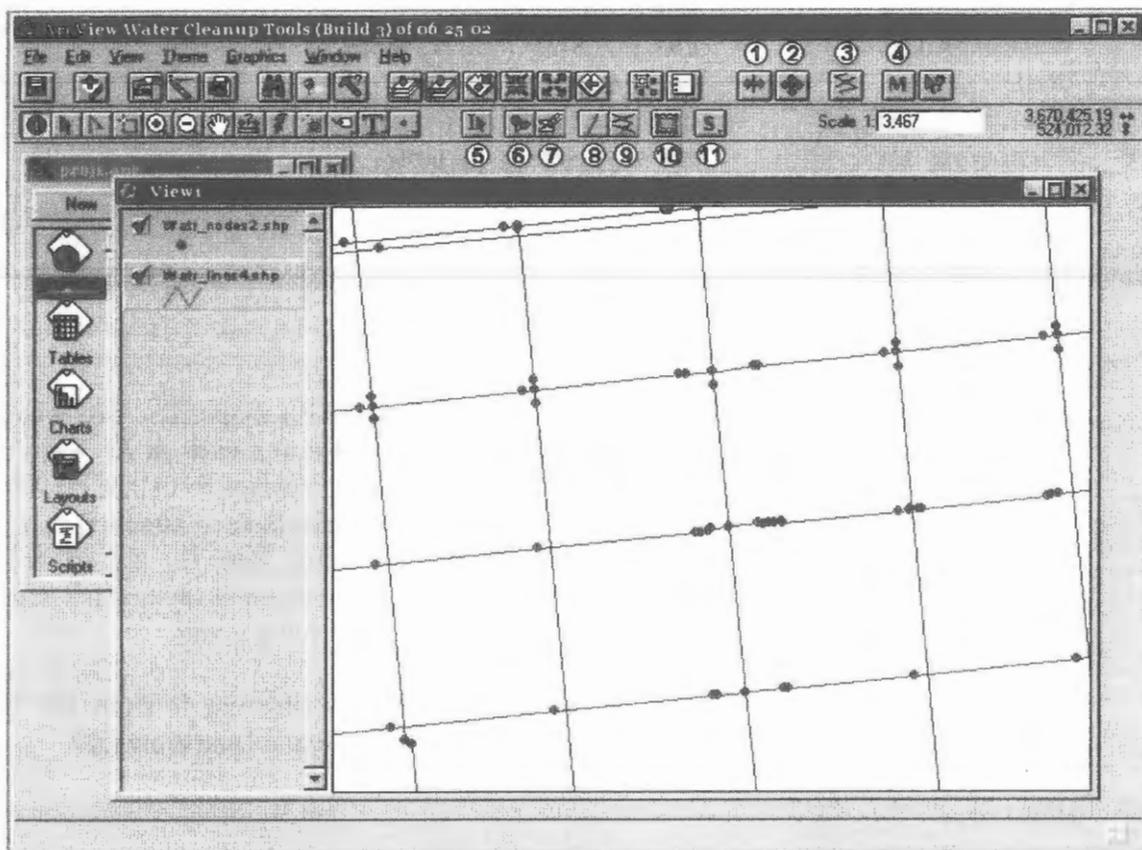
1. **Valve Trace** - Select the pipe(s) of interest and press this button to locate the valves that would need to be closed to isolate the pipe(s).
