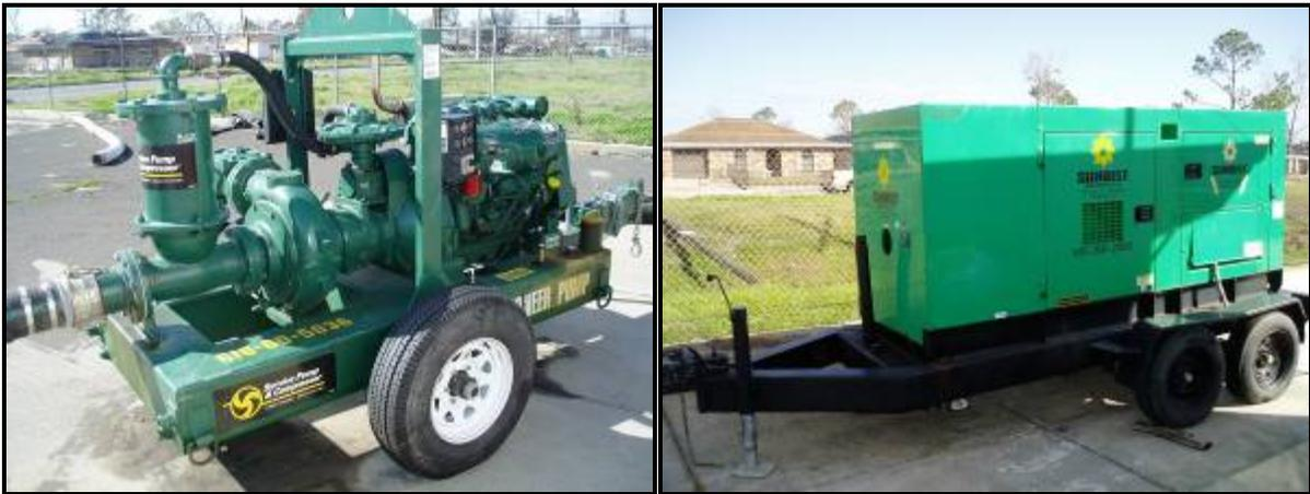
**Figure 11. Portable Pumps & Generators**
