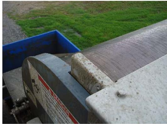
**Figure 7. Drum Screen for Grease Removal**
