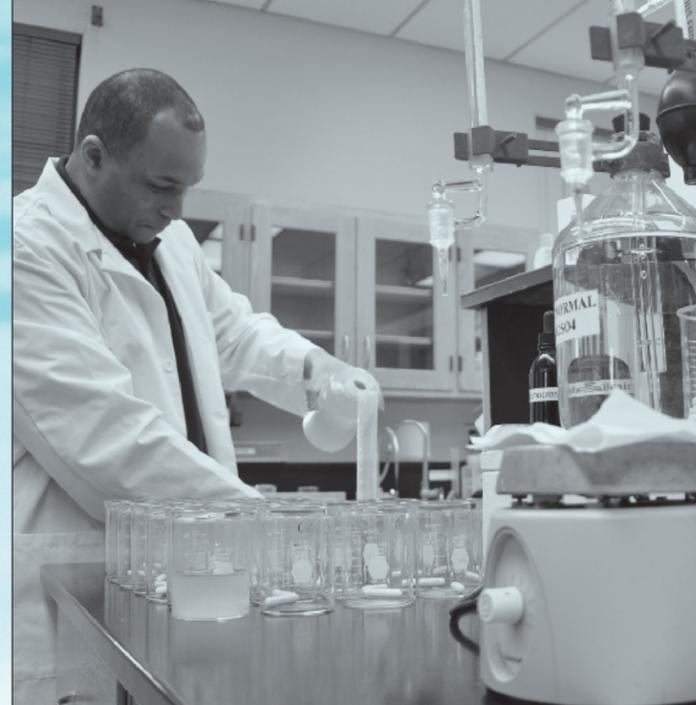
Staffed by chemists, microbiologists and technicians, the Sewerage and Water Board Water Quality Laboratory assures the safety and purity of the city's water by testing for organic, inorganic and microbiological compounds. The 8,500 square foot lab is located within the Carrollton Water Purification Plant and monitors river water and finished water sampled from both the East Bank and Algiers. Pictured here, a Laboratory chemist performs water analysis.
