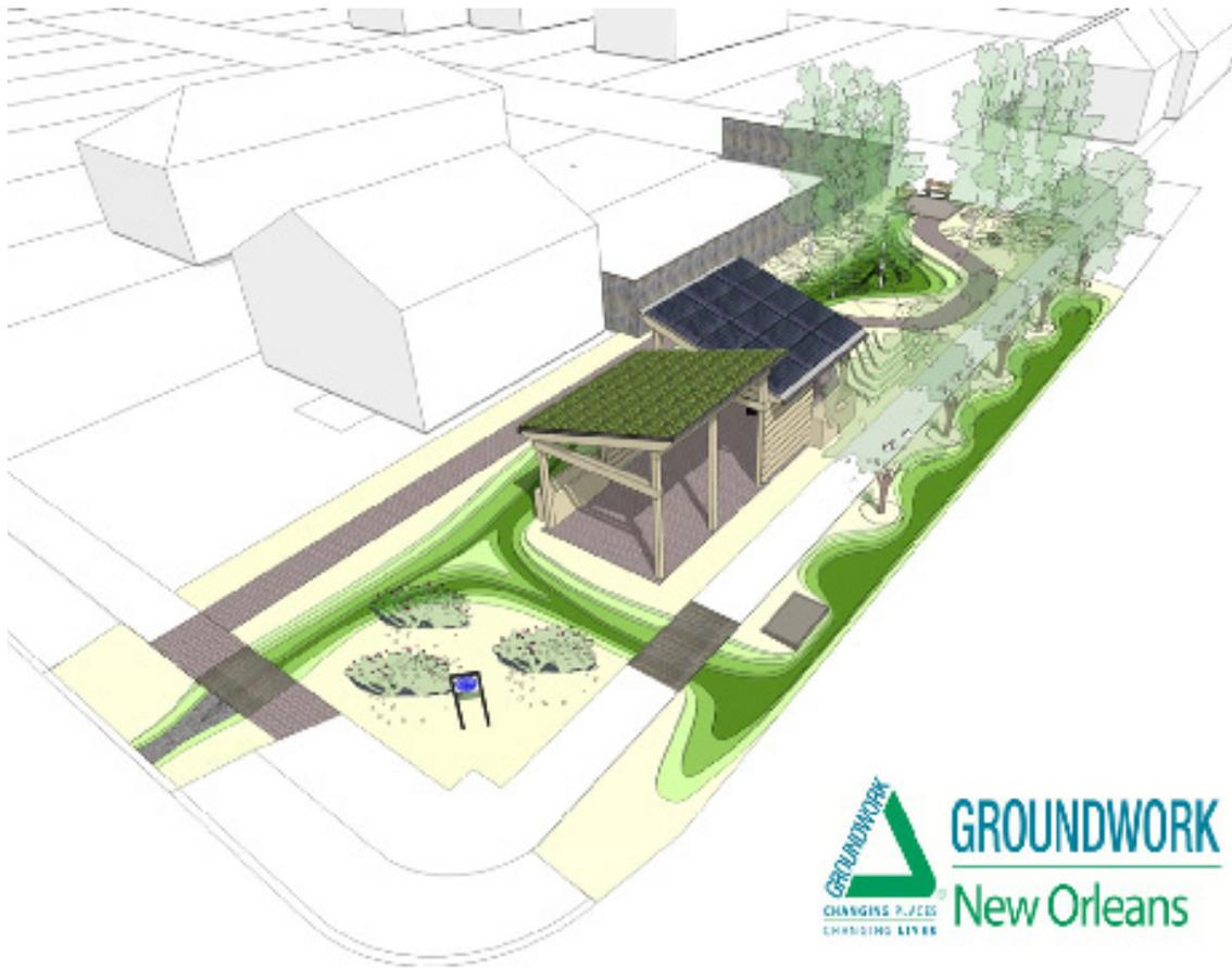
Earth Lab which includes a rain garden, bioswale, green roof, pervious pavement, stormwater quantity and quality monitoring equipment, and groundwater monitoring; development of a curriculum for high school students and a neighborhood adaptability model; and professional development workshops for neighborhoods, community groups, residents and professionals.
