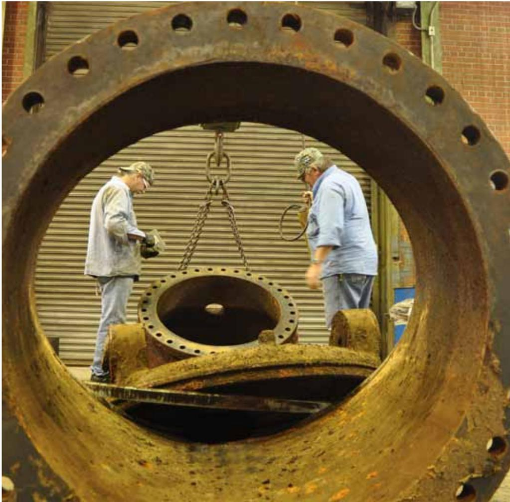
The Facility Maintenance Department fabricates, in-house, gears of various dimensions and specifications to accommodate the many different size valves that are used throughout the water and sewer systems.
